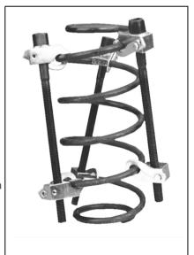
Tighten the spring compressor to compress the spring using equal pressure from each clamp, ensuring that the spring remains straight. If the spring starts to bend to one side, correct this by tightening the slackest side.
